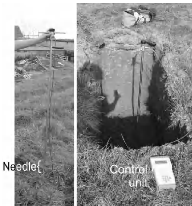
Figure 15.10 An example of a thermal needle probe being used to measure local in situ subsoil thermal conductivity in a 1-m-deep trial pit. Photo by David Banks.
