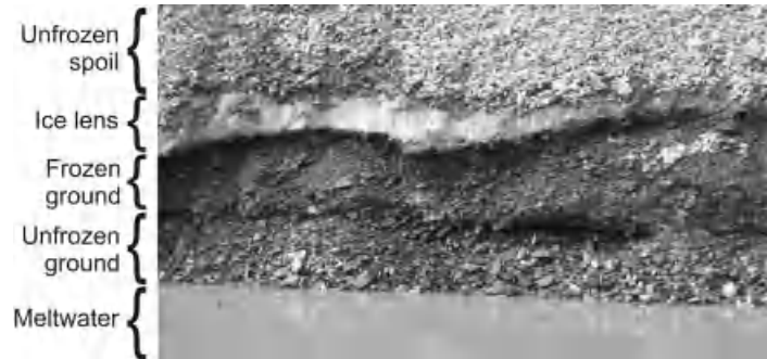
Figure 3.4 Frozen mining spoil at Novii Berikul in south-western Siberia. Frozen ground, formed during the previous severe winter, has persisted as a layer, over 1 m thick in places, well into August 2010, when the photo was taken. The frozen ground was exposed by excavators, extracting the mining spoil for use in road construction. Remember that this is not permafrost – it is seasonal frozen ground, which melts throughout the summer and autumn and which is sandwiched between unfrozen ground above and below. It clearly illustrates the fact that the ground is a highly efficient store of winter cold. Photo by D. Banks.
